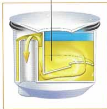
UNIQUE CARTRIDGE DESIGN REQUIRES NO ADDITION OF SEALANT BETWEEN CHANGES ...SECURELY ISOLATED FROM THE RESTROOM, WHILE PROCEEDING TO THE DRAIN
